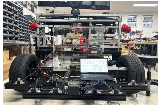
Fig. 3. Test-bed for LIN-CAN frames co-analysis
